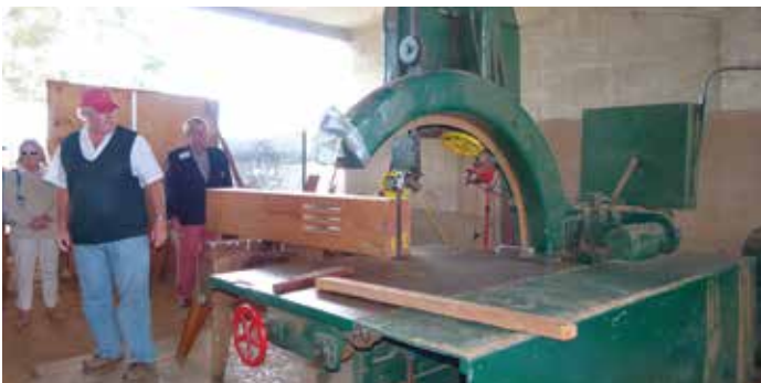
One on eight Ship's saws in the US, where the table remains flat while the blade angle can be changed
