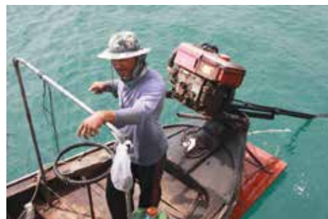
Longtail taxis with a gas engine and tiller; no reverse!
