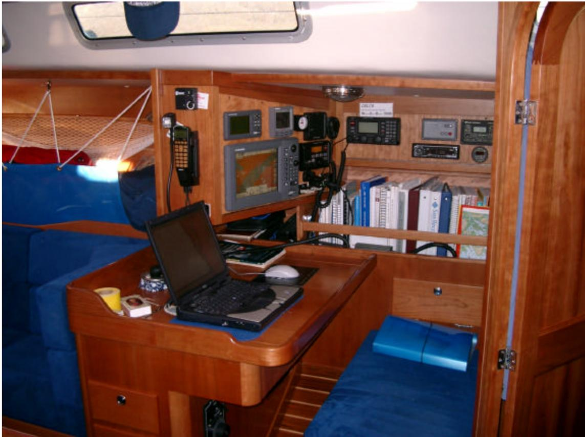
The chart table is equipped with a complete array of contemporary instrumentation including a Dell Inspiron laptop computer, Iridium satellite phone, Furuno Navtex, Furuno NavNet plotter and radar, Raynav instrument readout, Icom VHF radio transceiver, Icom SSB HF radio transceiver, Mastervolt genset controls, AM/FM stereo CD player, and electrical system monitors. Not seen on the bulkhead behind the navigator is the entire circuit breaker panel.
