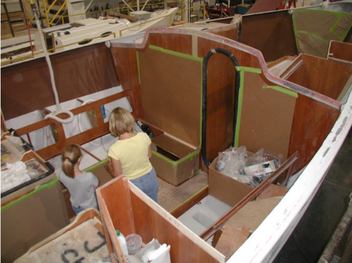
View of the main cabin during construction. The main bulkhead was fitted with a watertight door and silicone seals were installed on all wiring and plumbing passing through this bulkhead.
