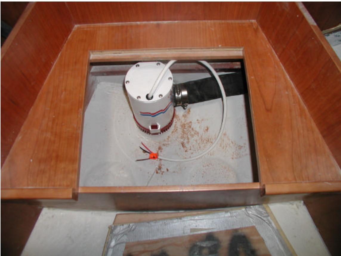
High-capacity bilge pump installed in the forward cabin
