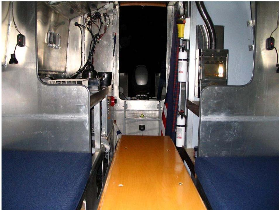
The galley and enclosed head are adjacent to the companionway. Note the propane cabin heater and multiple fire extinguishers.
