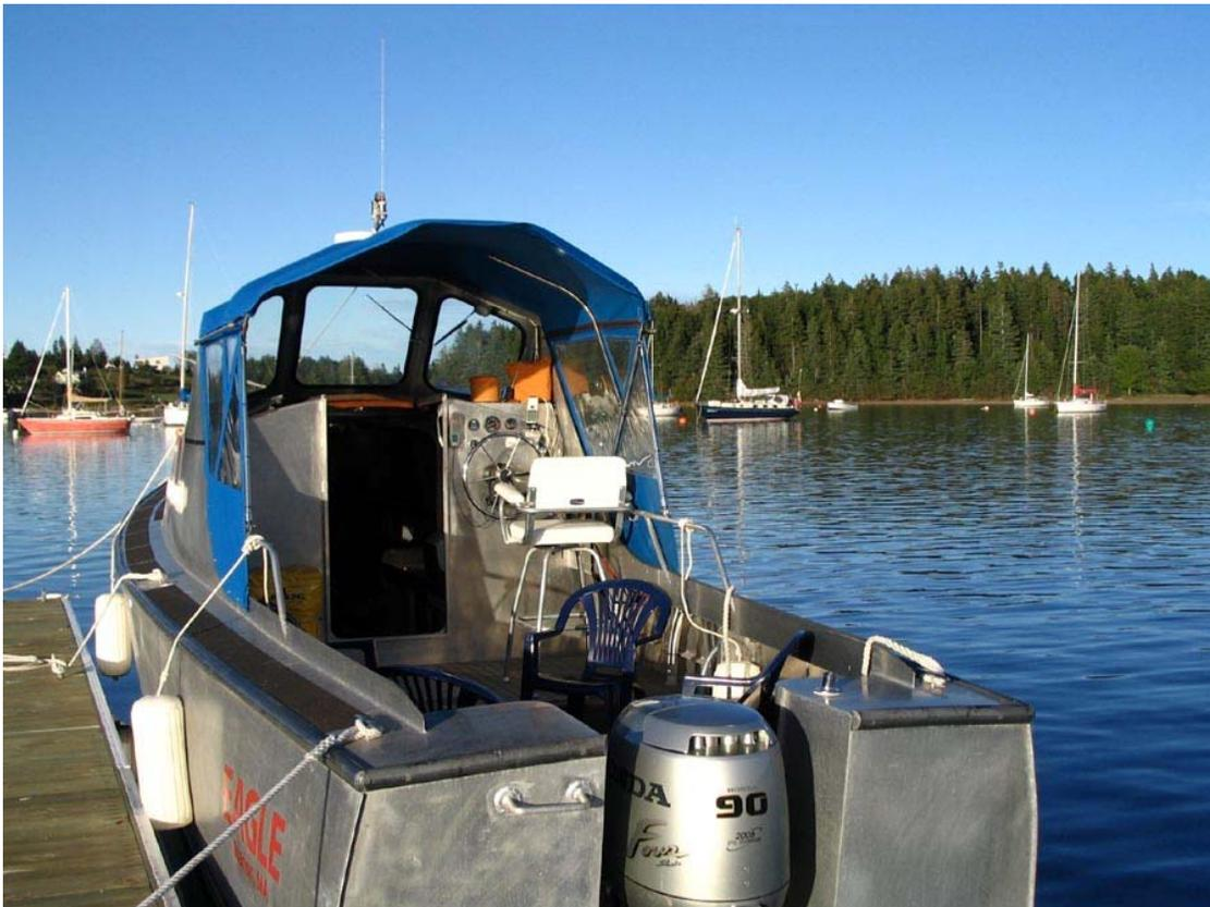
This view from astern shows *Eagle's* cockpit, steering station, and engine arrangement.
