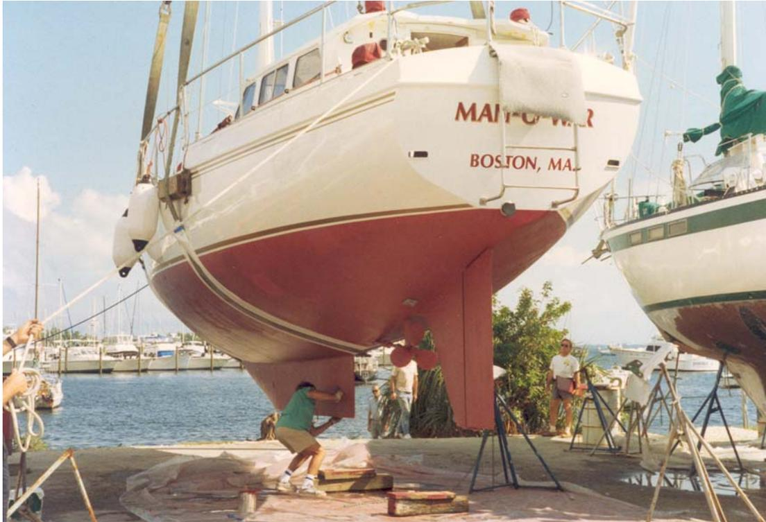
The full underbody provides room for the 300 US gallons of fuel in four integral tanks and 300 gallons of water in six integral tanks. The short box keel contains the DC electric driven centerboard as well as space for pumps, fuel filters, etc.. The skeg hung rudder is strong enough to have split a coral head while backing off Light House Reef in Belize.
