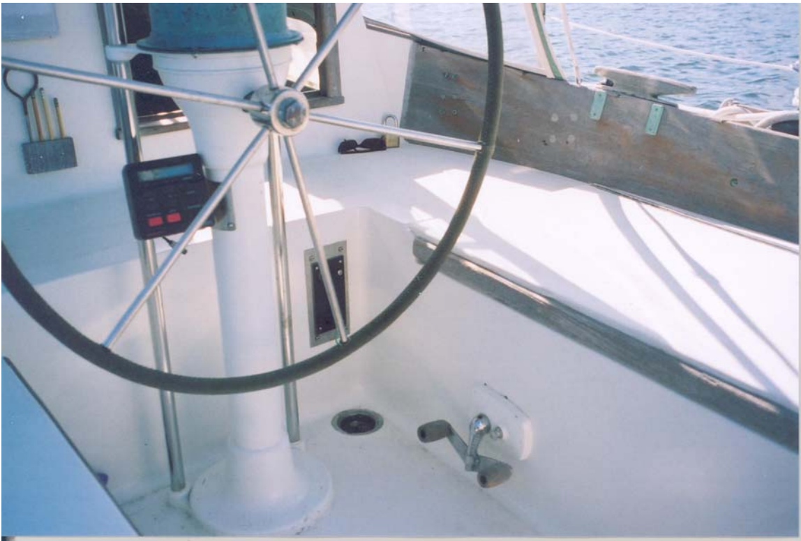
The novel foot pedal actuates the throttle and reverse gear.
