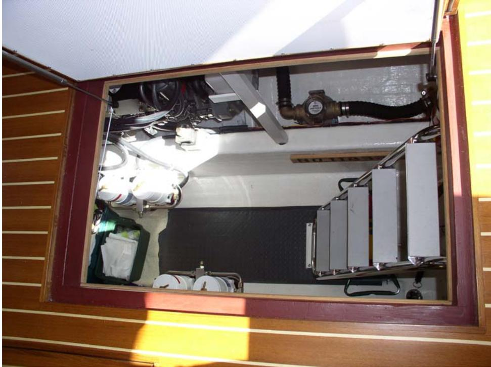
Looking down into the spacious engine room through the counter-balanced hatch at the forward end of the main cabin sole.
