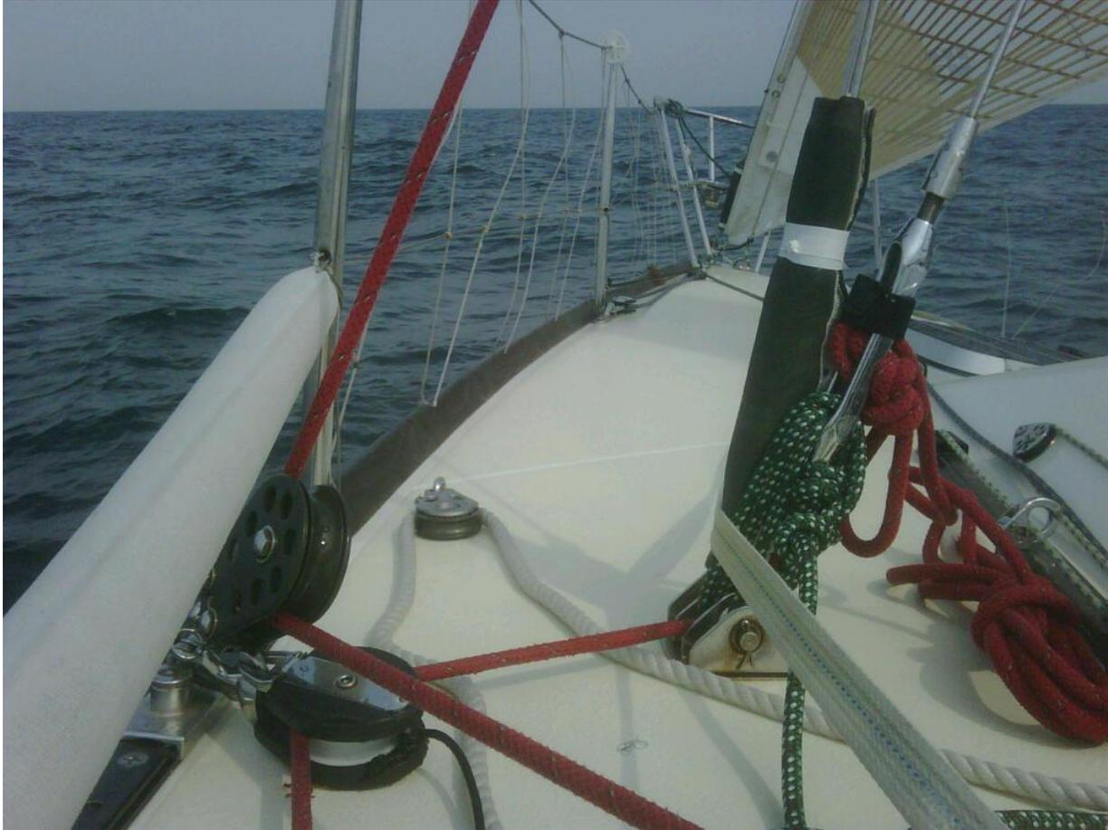
Picture 3 . The red line leading through the block flat on the deck tensions the shroud. The second red line leads to the mast at the spreaders and provides further support.
