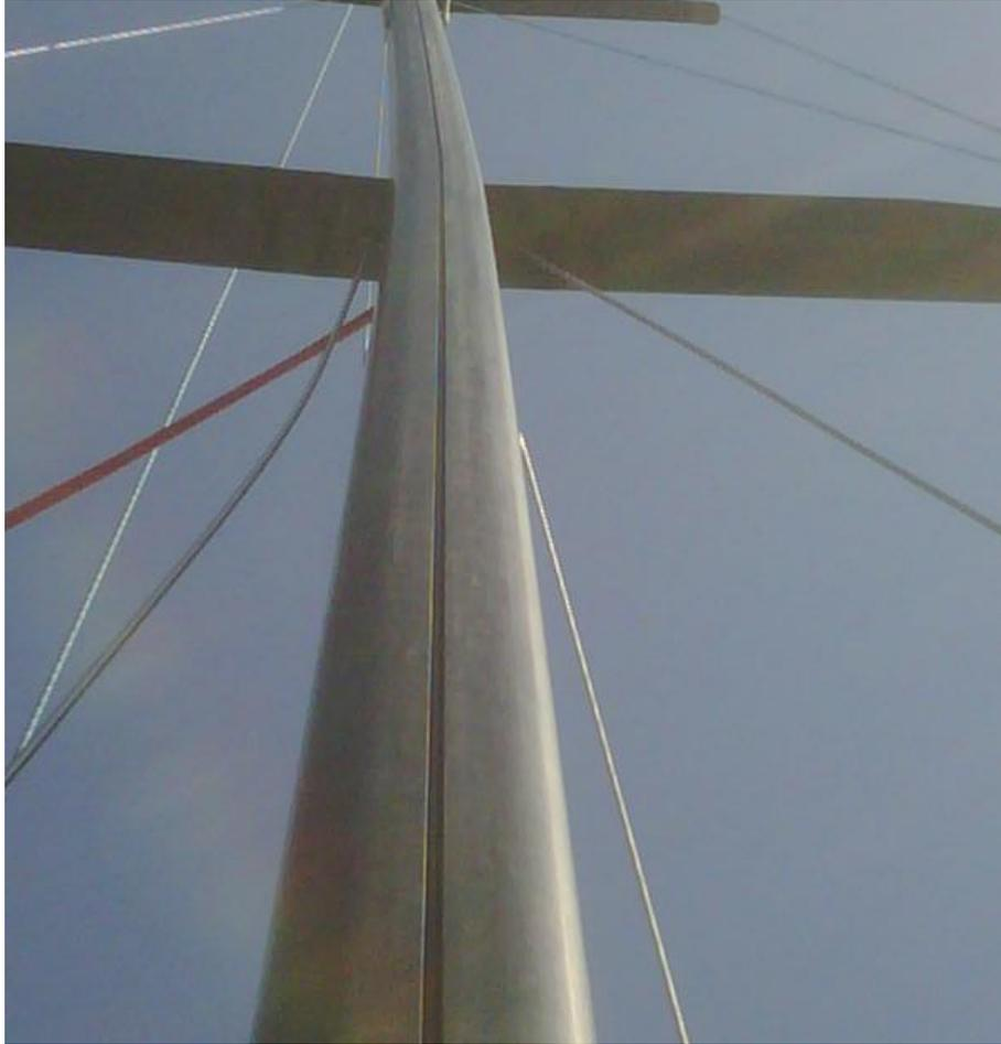
Picture 4 The mast, taken from behind. Shows the bend in the mast after we minimized the bend by leading a masthead halyard under the convex side of the bend and up to port, then winching the mast back into column. Note supplementary shroud (red line) that we led once seas had calmed.
