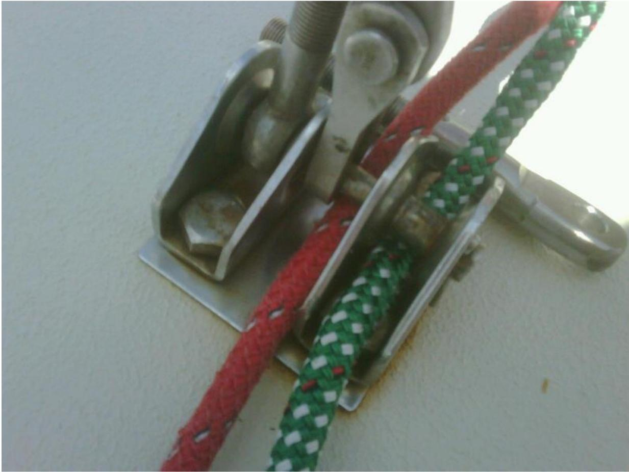
Picture 2 The green line is a strop rigged immediately to connect the turnbuckle to the chain plate. The red line was also attached to the turnbuckle, then led aft to a winch to tension the repaired shroud.
