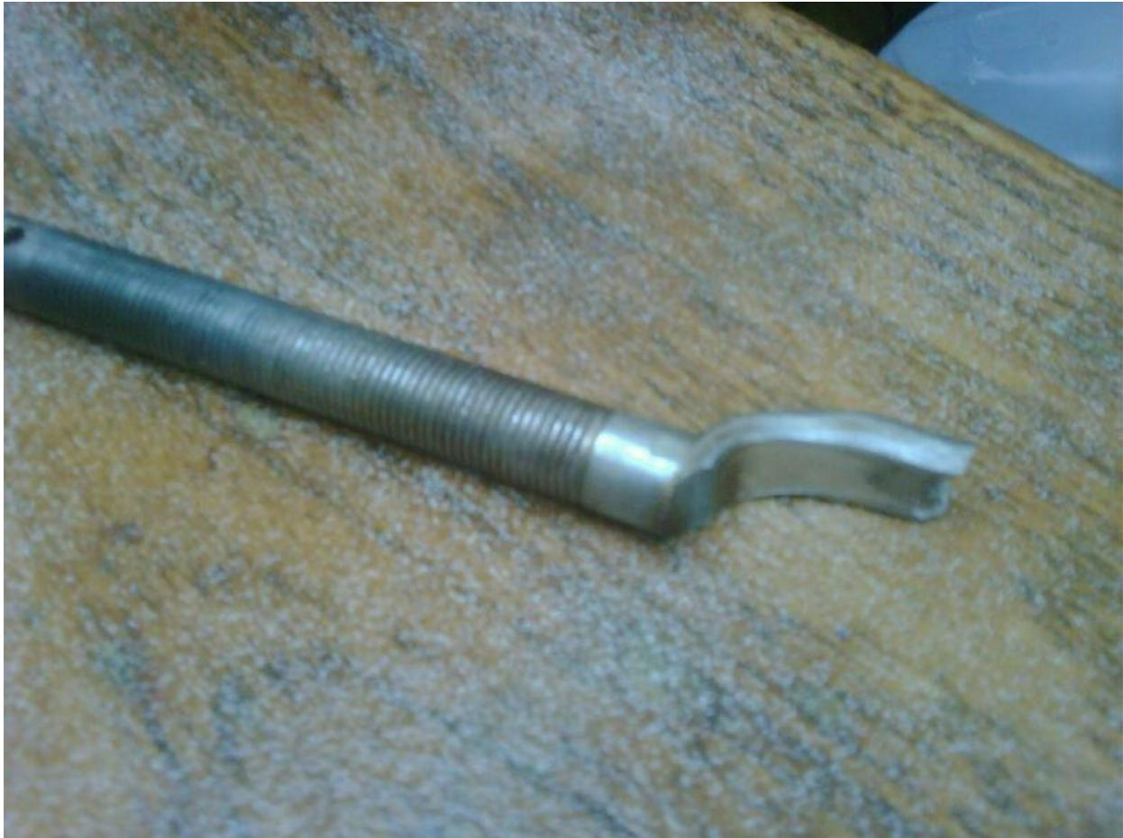
Picture 1 Bottom of turnbuckle on lower port shroud showing where the forging cracked.
