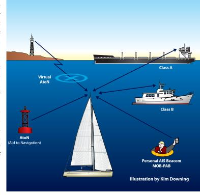
transceivers. Some boats have receive-only AIS without a transmitter, enabling them to 'see' others though they cannot be 'seen' themselves. In low visibility conditions with lots of AIS targets, it is easy to assume that every boat has AIS but other means, such as radar and listening, should always be used in addition to AIS to prevent collisions.
