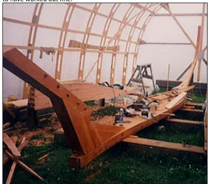
The deadwood was sandwiched together from more of the fir planks using asphalt roofing cement between layers and many long 5/8" bronze bolts. Stern post, horn knees timber, transom frame all came from the pile of black locust.
