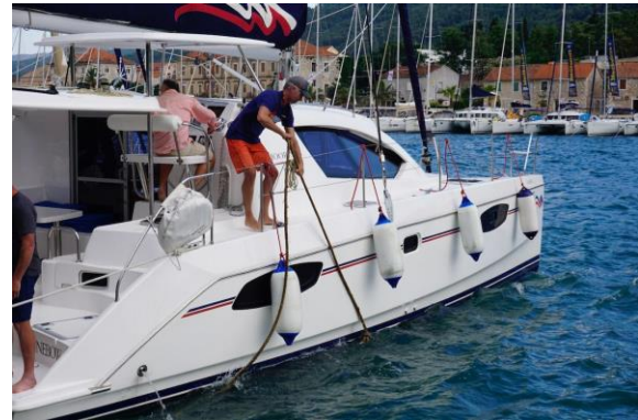
A dockmaster on the seawall hands you lines which connect to concrete blocks underwater. Very secure, and no need for anchors.
