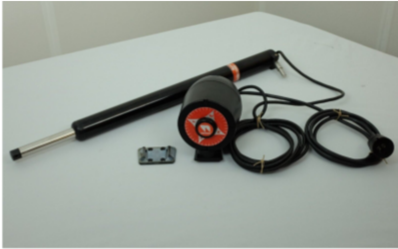
The original version of the Autohelm 2000 autopilot. Note the small actuator and the separate compass/electronics.
