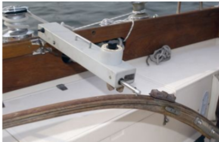
Example of a Tillermaster installation. Note that gravity is largely responsible for holding the autopilot in place. Mark Corke photo.
